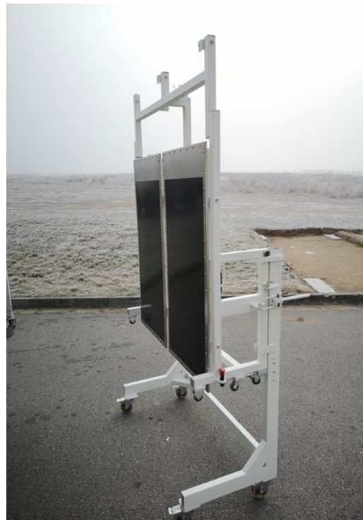
Fig. 2 A side view of the storage space of the van (left) with the detectors installed in the measuring position; a pair of detectors taken out of the vehicle (right) for measuring the geometry of the corridor
