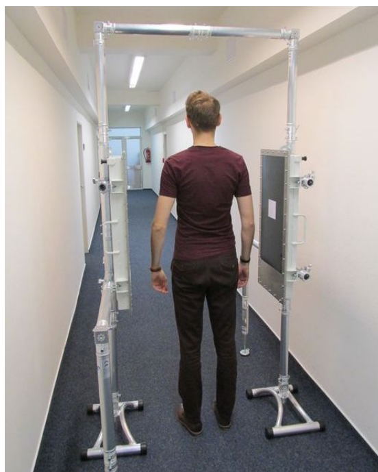
Fig. 4 "Mobile portal detector - passenger car" when measuring people in the corridor configuration
