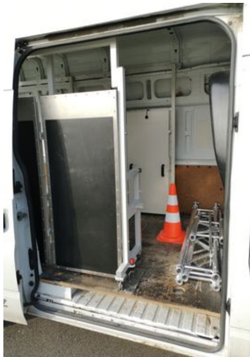
Fig. 2 A side view of the storage space of the van (left) with the detectors installed in the measuring position; a pair of detectors taken out of the vehicle (right) for measuring the geometry of the corridor
