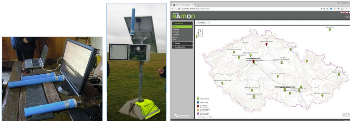
Fig. 4 MOSTAR - detectors (standard and stand-alone), web presentation of results
