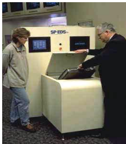
Fig. 4: Checking a case with the TNA method, using the appliance of SPEDS from the company called Ancore. 2
