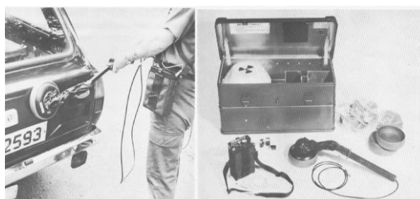
Fig. 1: The detector of explosives HED L3A1, the first and most recent neutron detector of explosives used in the Czech and Slovak Republic 4
