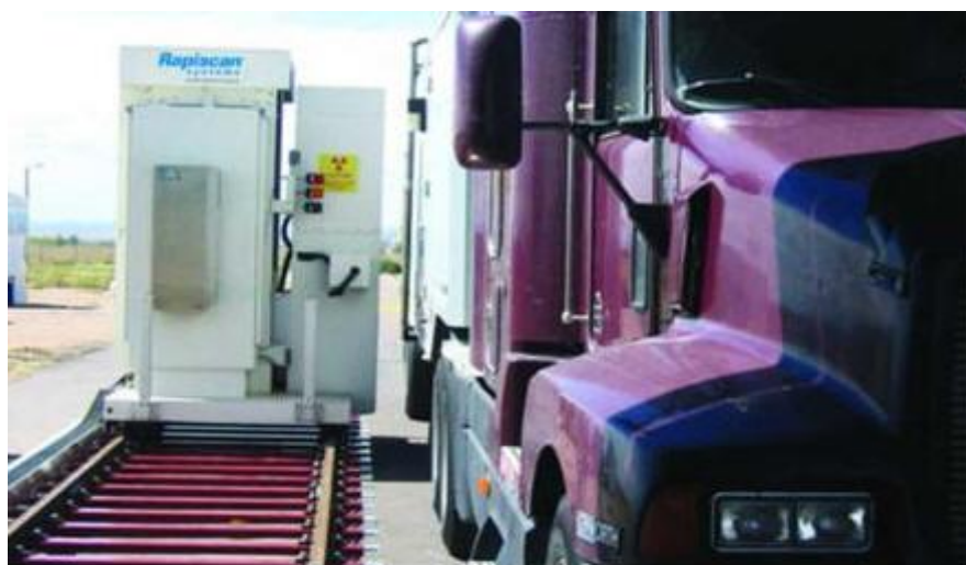
Fig. 5: Customs inspection done by a combination of methods TNA and FNA – system VEDS (Vehicle Explosive Detection System). 2
